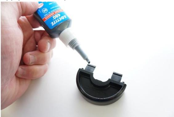
Place a small drop of Loctite 480 in each standoff tine groove prior to assembly.
