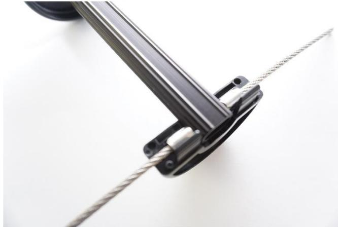
4. Place additional standoff halves on top of standoff halves supporting ladder rung, apply light pressure until the halves snap together. **NOTE: It may be necessary to apply tension or a slight twisting motion to rope ladders to stop the halves from pinching rope during assembly.**
